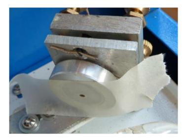
Once the mirror is positioned, ensure all the screws are tightened, remove the masking tape and clean the mirror to remove the burnt residue of masking tape.
