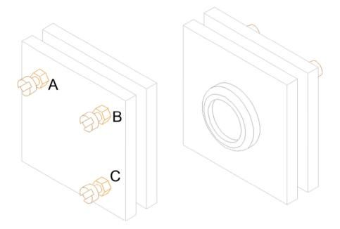
The picture above shows mirror adjusting assembly. The three screws A, B & C are locked with lock-nuts. These should be treated with care - the screws and nuts are brass and have a fine pitch thread. Too much enthusiasm will result in stripped threads probably requiring a new mirror assembly.
