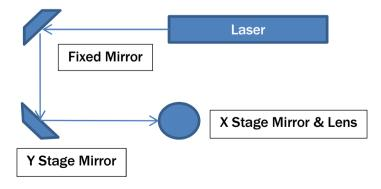
The laser lies parallel to the X axis of the X-Y stage, The beam is reflected onto the Y axis by the fixed mirror and then back onto the X axis by the Y stage mirror. The X stage mirror then reflects the beam so it is vertical and through the lens.
