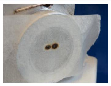
In an ideal world, the two spots will be on top of each other. In practice there will be two spots. The relative position of the two spots tells you how to adjust the mirror. If you cannot see the second spot because the fixed mirror is too far out of adjustment, move the Y axis mirror a smaller amount at first until the alignment is close enough that two spots can be produced when the Y axis mirror is moved over its full travel or the spots are aligned.
