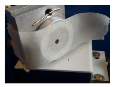
A well-adjusted fixed mirror and correctly positioned Y axis mirror will give a result as above. Once this has been achieved the Y axis mirror can be aligned.
